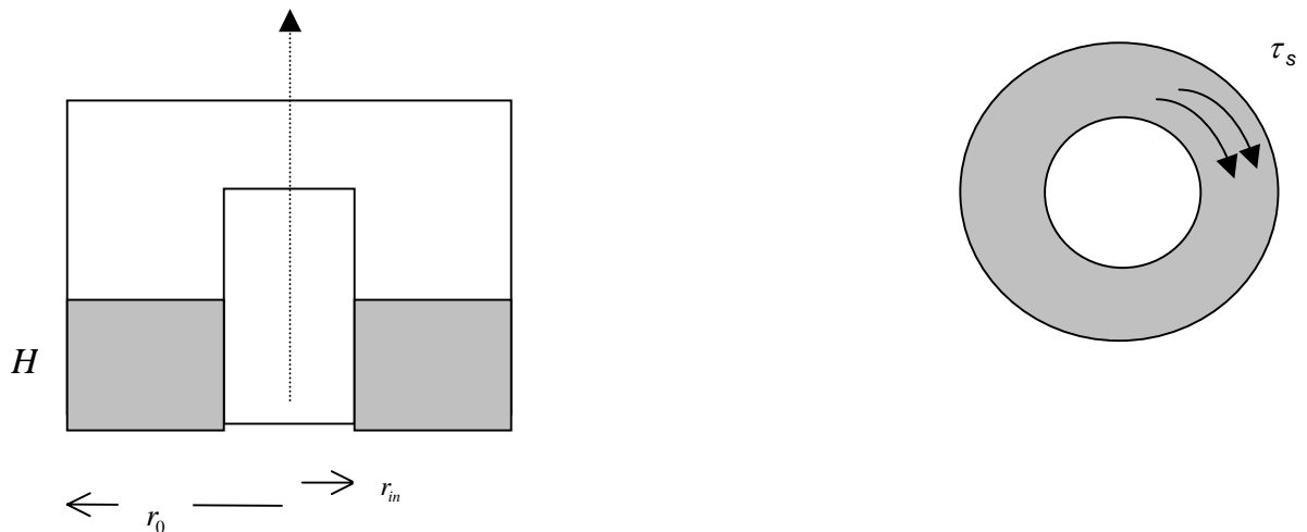
Figure 3: Side and upper views of the wind wave tank. Air motion over the water surface results in a propelling shear stress \tau_s and propelling torque T_{propel} .
