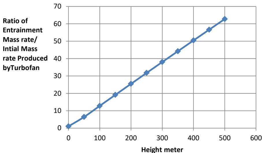
Figure 4: Jet mass flow rate due to entrainment. Turbofan initial mass flow rate is 705 kg sec<sup>-1</sup>.
