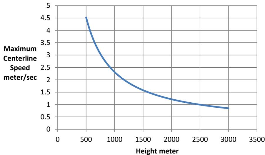
Figure 3: Jet Maximum Centerline Velocity Vs. Height; Initial Jet Velocity 143 meter/sec.
