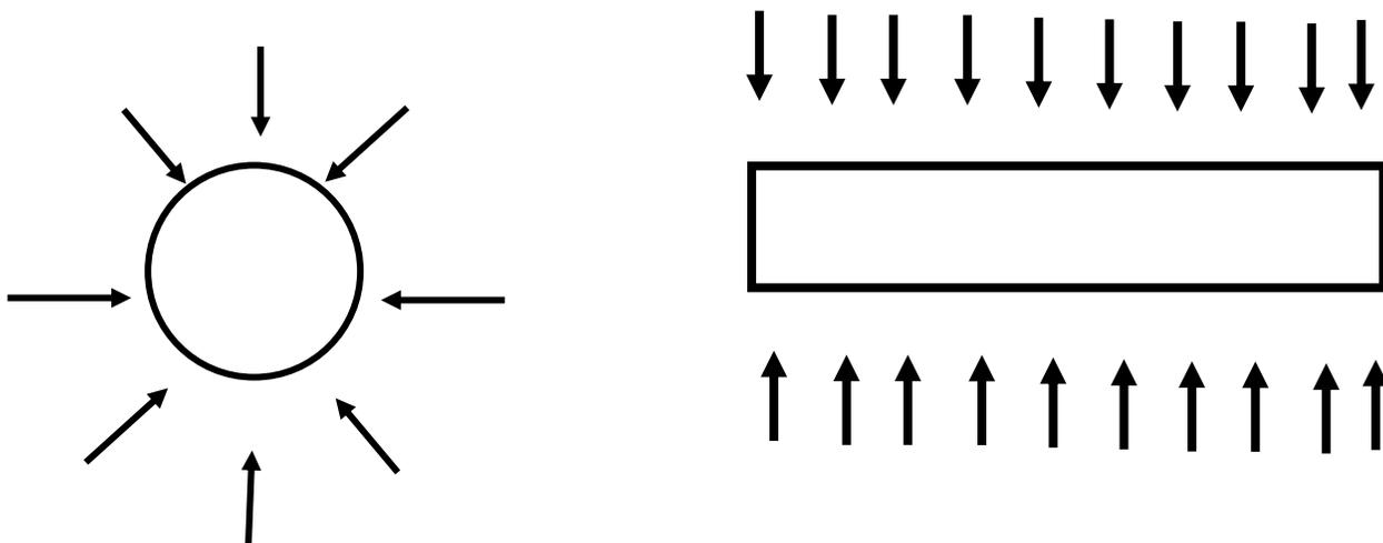
Figure 10: Entrainment into circular jet versus planar jet.
