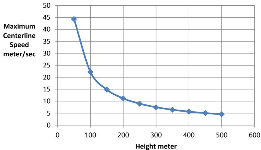
Figure 2: Jet Maximum Centerline Velocity Vs. Height; Initial Jet Velocity is 143 m/sec.
