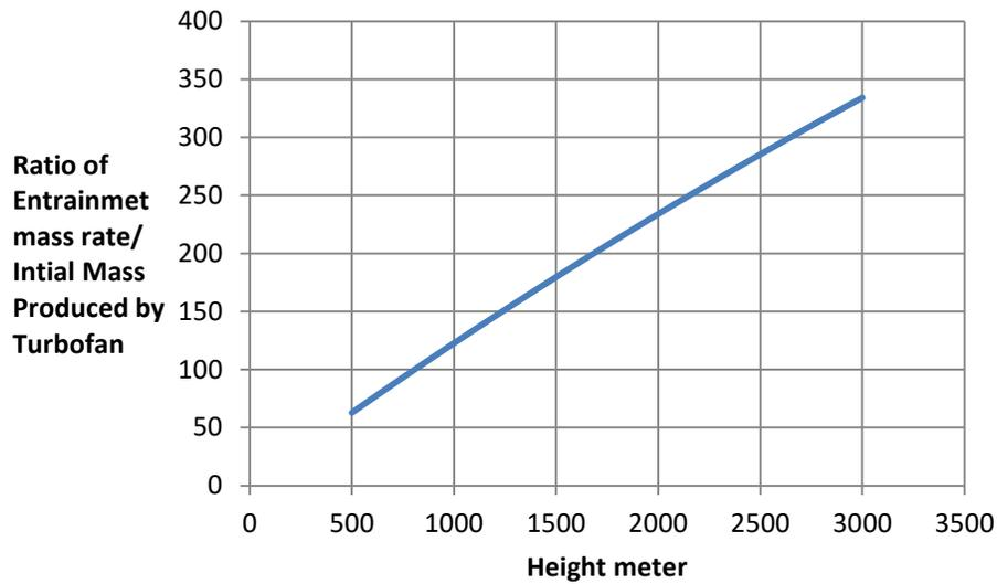
Figure 5: Jet mass flow rate due to entrainment. Engine initial mass flow rate is  $705 \text{ kg sec}^{-1}$ .
